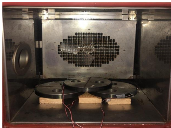
Figure 2: Carbon Fiber Composite in Climate Chamber
